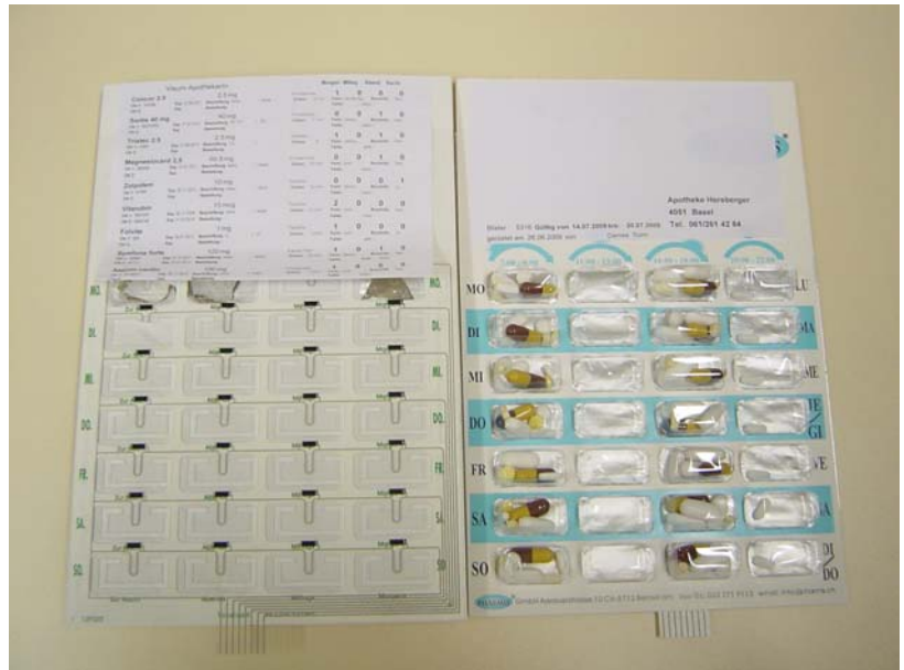
Figure 1a (left): electronic foil with conductive tracks, battery and antenna fitting a commercially available blisterpack (Confrérie Clinique S.A., Lausanne, CH.). Figure 1b (right): Vinalink® blisterpack (Pharmis GmbH, Beinwil a.S., Switzerland) with conductive loops of electronics on its backside (film side) covering the 7x4 cavities prefilled with patient's individualized medication regimen (front side).
